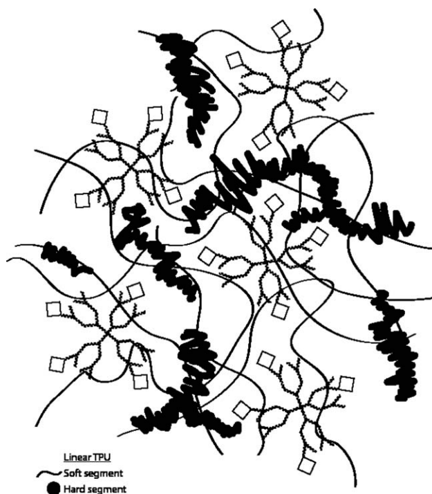
Figure 6 Distribution of POSS-functionalized Boltorn throughout the soft (polyester) segment within TPU.
